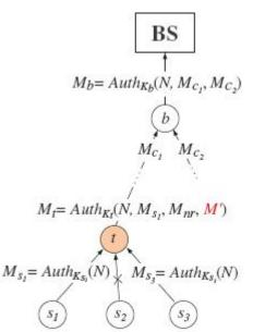
Figure 4 ALS.I: Hierarchical Collection of Confirmations *Recursive Processing of Confirmations:* The above procedure results in message Mb reaching the BS. If no message is received, then b, the single child of the BS, is marked. Otherwise, the message is processed in a recursive manner. As the aggregation tree is known to the BS, it knows that Mb should be authenticated using Kb. If it is, and the message begins with N, and the proper number of *child* messages (equal to the number of b's
